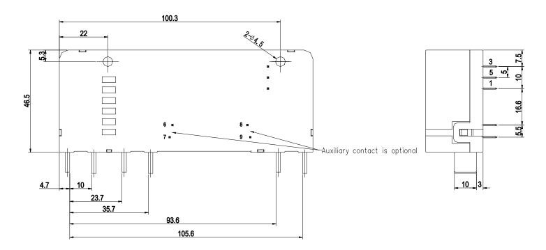
Remark: (1) In case of no tolerance shown in outline dimension:outline dimension≤1mm,tolerance should be±0.2mm;outline dimension>1mm and <5mm,tolerance should be ±0.3mm;outline dimension≥5mm,tolerance should be ±0.5mm.
