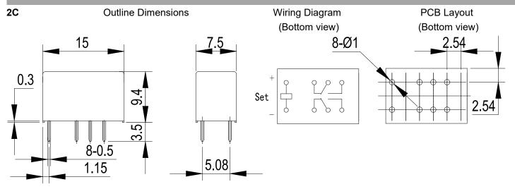
Remark:(1)In case of no tolerance shown in outline dimension:outline dimension≤1mm,tolerance should be±0.2mm;outline dimension>1mm and <5mm,tolerance should be ±0.3mm;outline dimension≥5mm,tolerance should be ±0.5mm.
