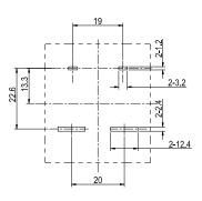
Remark:(1)In case of no tolerance shown in outline dimension:outline dimension≤1mm,tolerance should be±0.2mm;outline dimension>1mm and <5mm,tolerance should be ±0.3mm;outline dimension≥5mm,tolerance should be ±0.5mm.
